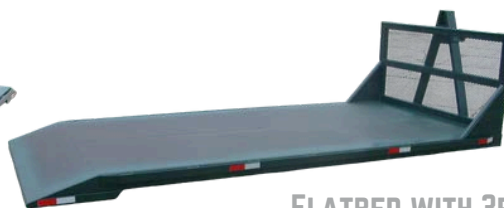
FLATBED WITH 3FT BEAVER TAIL & EXPANDED METAL BULKHEAD
